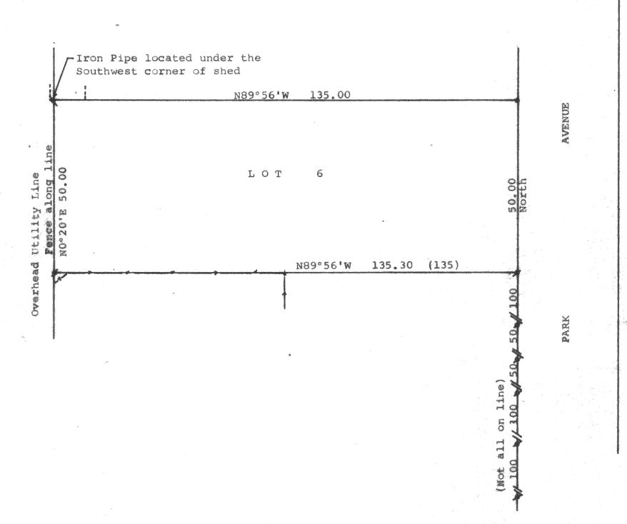
Scale - 1" = 20' N= 3/4" X 24" Iron Pipe Set e= 1½" X 24" Iron Pipe Set ≠= Iron Pipes or rods found (0.00) = recorded distance Bearings referenced to the west line of Park Avenue with the assumed bearing of North
